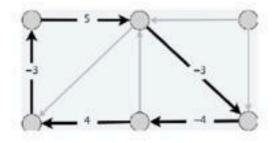
**Lemma 2**. If G has no negative cycles, then there exists a shortest  $v \leadsto t$  path that is simple (and has n – 1 edges).
