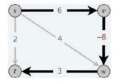
**Re-weighting**. Adding a constant to every edge length does not necessarily make Dijkstra's algorithm produce shortest paths.
